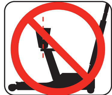
The load should be centrally located on the head cap.
