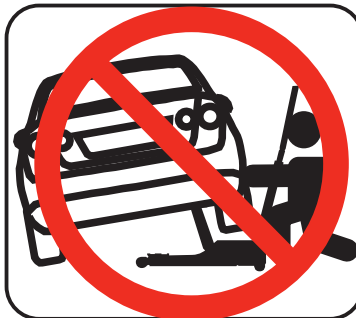
This hydraulic trolley jack should be used for lifting and lowering only; The raised vehicle should be supported on two vehicle support stands.
