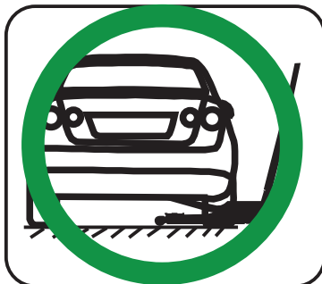
Personal protection equipment is required before operation. The unlifted wheels of the vehicle should be chocked.
