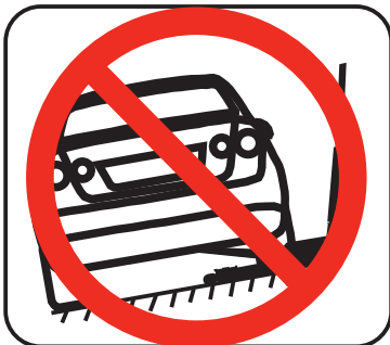
The trolley jack should be used on a hard level surface and be free to roll during lifting and lowering.
