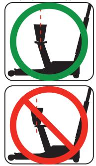
The load should be centrally located on the head cap.
