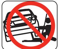
This hydraulic trolley jack should be used for lifting and lowering only; The raised vehicle should be supported on two vehicle support stands.
